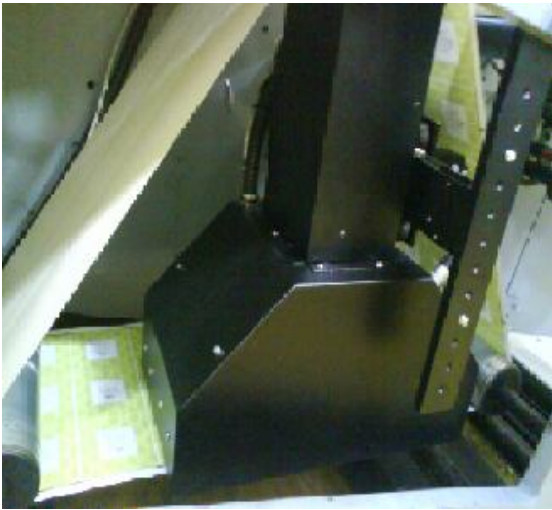
T shape camera housing installed on an MPS press
