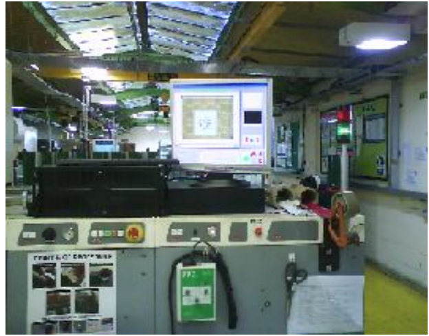
AVIS system with print defect detection installed on MPS press
